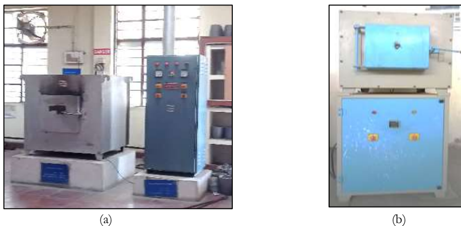
Figure 2: (a) 18 KW Electrical Furnace coil type for melting (c) 3KW box type muffle furnace for preheating
