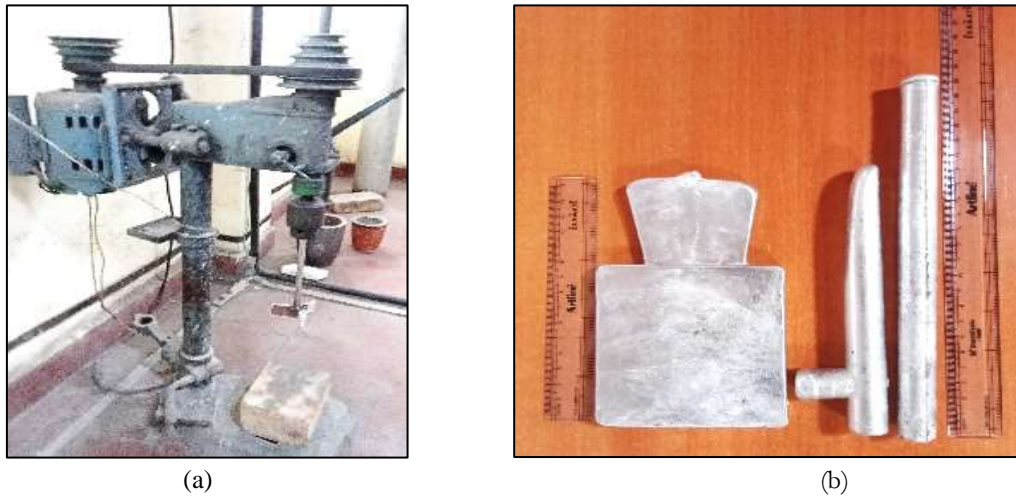
Figure 3: (a) Stirring machine (b) Fabricated composites
