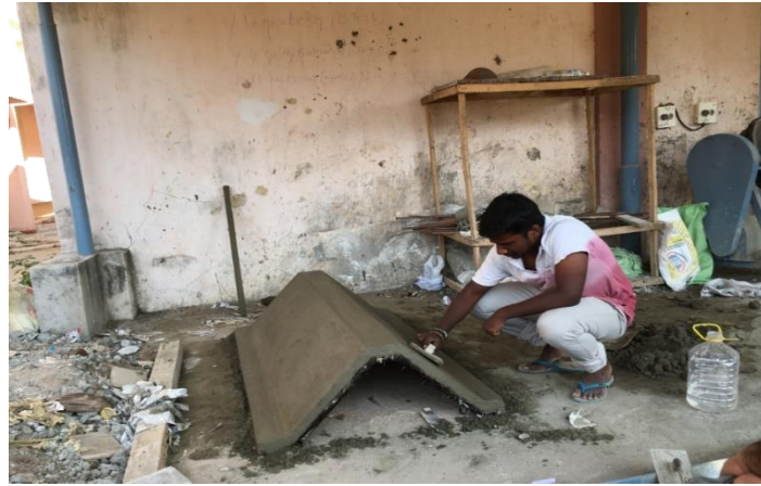
Fig 6: Casting of Specimen Coved Ferrocement
