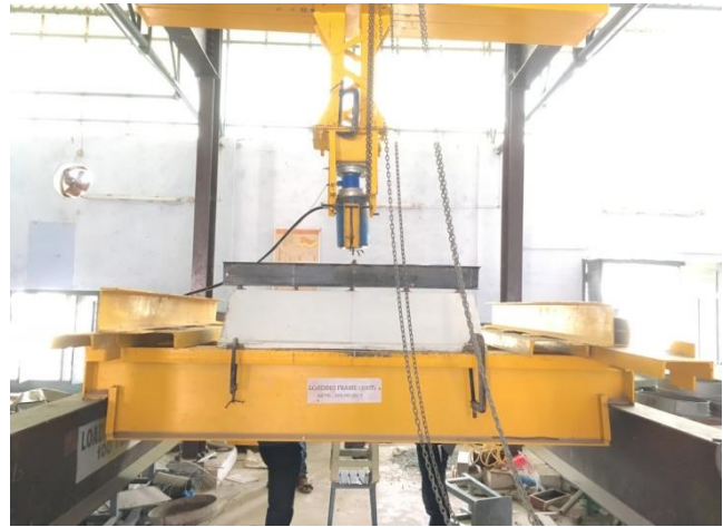
Figure 8: During Testing of Ferrocement Folded Plate
