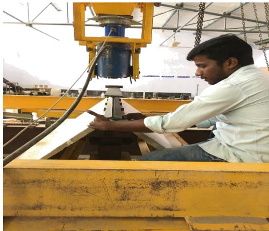
Figure7: Placing of Specimen on Loading Frame
