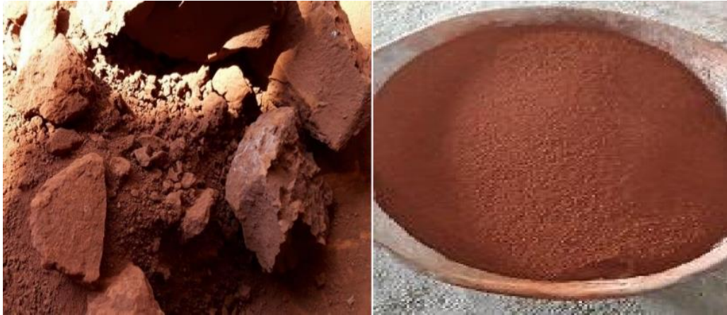
Figure 2: Raw iron ore tailings and crushed iron ore tailings
