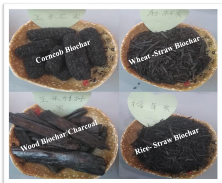
Figure 3: shows the four types of biochar that were produced from (a) Corncob, (b) Straw of Rice, (c) Woods, and (d) Straw of Wheat. These images have been taken by Assistant Professor Gulaqa Anwari on the day of the international conference “First International Conformance on Biochar Research and Application” on September 20, 2019, in Shenyang Liaoning China.
