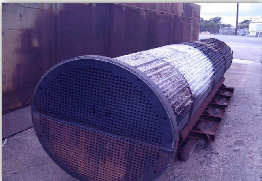
Figure 7: Heat exchanger bundles accumulated with popcorn polymers [6]
