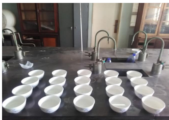
Figure 1: Illustration of the larvicidal assay showing bowls containing each 25 larvae in 250 ml solution for a given inorganic salt in five different concentrations (lines). Each concentration was repeated four times (columns)
