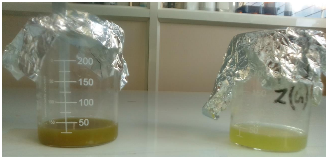
Figure 1: ZnO nanoparticles from green chillie extract
