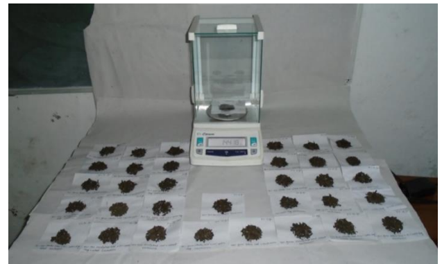
Figure 2: Measurement of moisture of vermicomposting and composting mixtures
