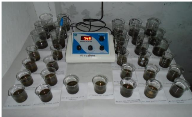
Figure 1: Measurement of pH using digital pH meter.
