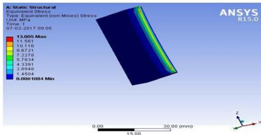
Figure 10: Analysis of cutting blades in ANSYS 15
