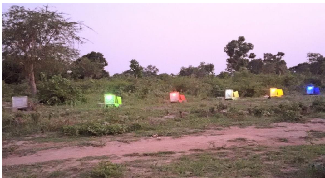
Figure 1: Fabricated light traps, spaced 3m apart used for sampling A. africana in the field
