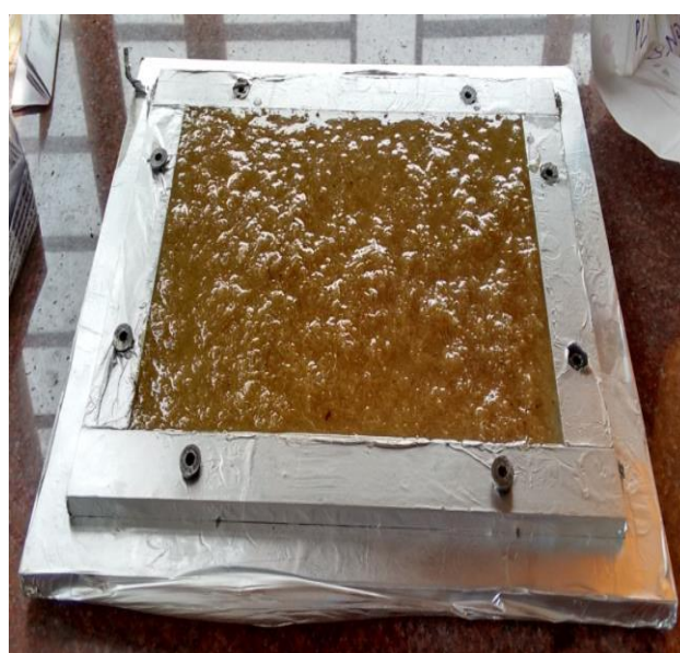
Figure 3: Moulds and sample preparation for mechanical testing
