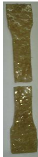
Figure 4: Tensile testing machine and Specimen After failure
